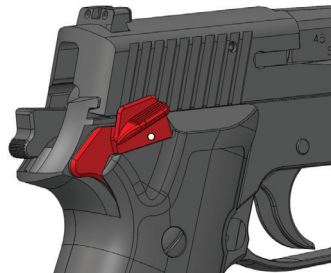
RIGHT SIDE MANUAL SAFETY ENGAGED
